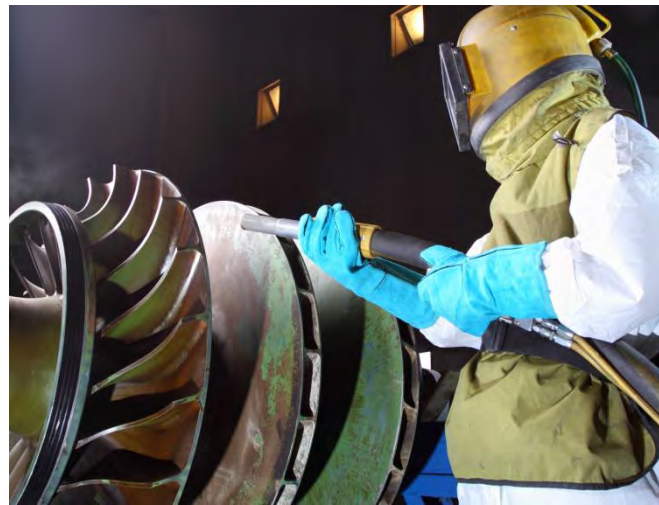
Contractor abrasive blast cleaning a steel component
