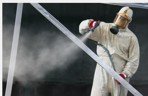
Spray painting results in a superior finish, but such coatings are generally high in VOCs and the method produces loss due to “overspray”
